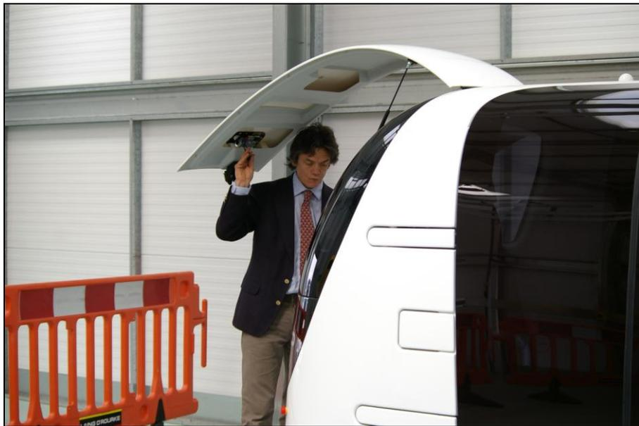
*Figure 1: Front of Vehicle Escape Hatch*
