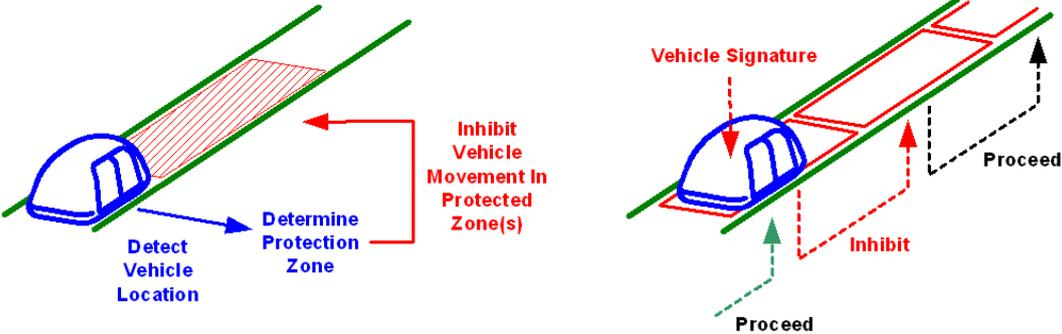
The AVP System employs redundant architecture so that single failures within any section of guideway do not result in any impact on operations or require that the safety system be completely switched off to allow continuing operations.
