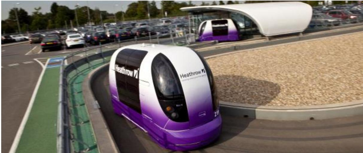
The vehicle is based on conventional automotive technologies and is electrically powered with four rubber tired wheels. Principal parameters are given in Table.
