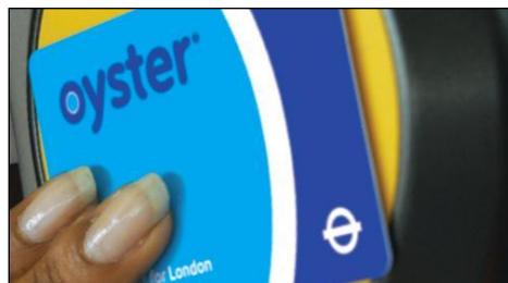
*Figure 1: Oyster Card being read at a fare gate with a touch to the "yellow card reader".*
