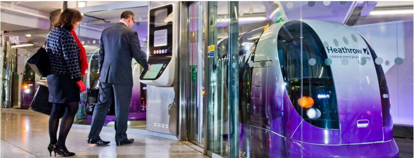
*Terminal station – Focal or terminal stations require multiple-berths that are typically within or attached to a host building. In such instances canopy and parts of the envelope may not be required but otherwise the same elements are employed.*
