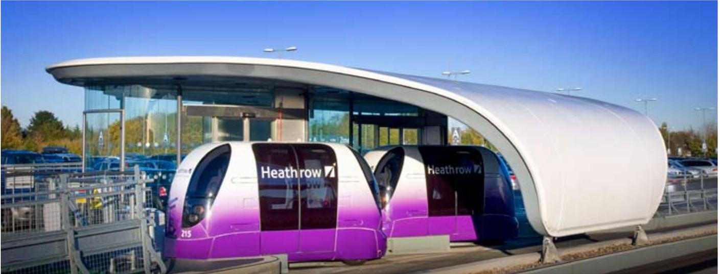
*Remote station – Comprises 20m<sup>2</sup> passenger weather-protected concourse and two berths; 1-berth and 3-or-more-berth versions are developed from the same elements.*
