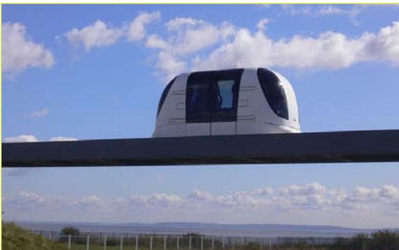
Ultra's pod system guideways are only 45cm deep (including kerbs), minimising their visual impact. Part of the reason for this is that the lightweight nature of the system gives it a low loading requirement; the British standard for a footpath is 5kN/m<sup>2</sup>, whereas the pods system is only 2.2kN/m<sup>2</sup>. This low overall loading also allows the vehicles to run on existing building floors without significant strengthening or modification.
