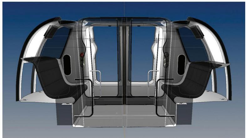
Ultra's pod interiors are customisable, with the vacuum-formed grey panels offering a neutral base onto which appropriate designs and graphics can be printed.
